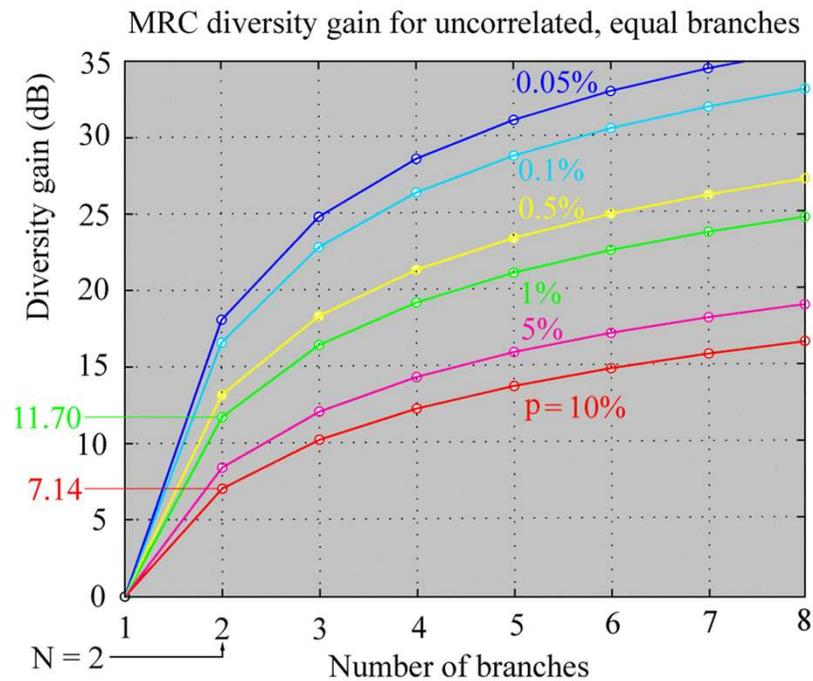
For a Rayleigh fading channel, the MRC diversity gain for un-correlated equal power branches is shown in the diagram.
