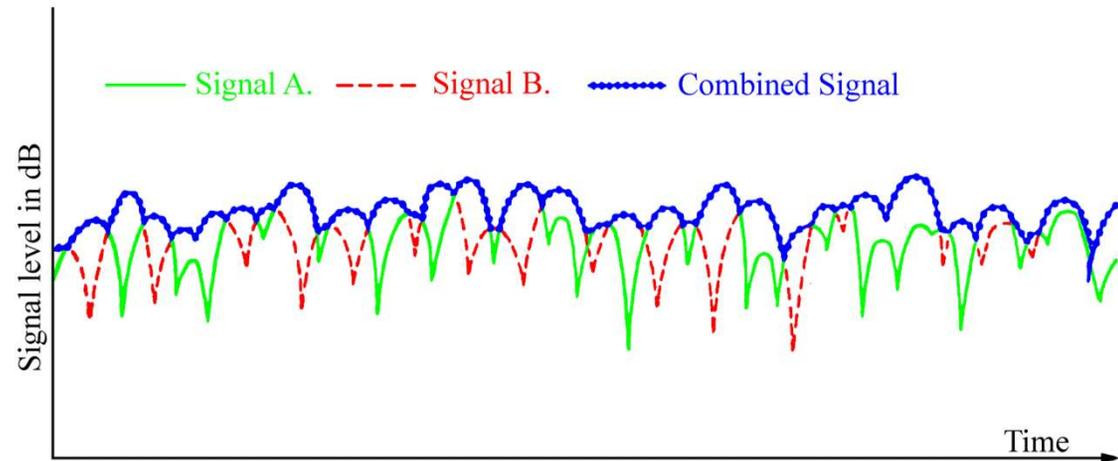
**Diversity gain** is defined as the improvement in the time-averaged **SINR** from the combined signals of a set of diversity elements, relative to the **SINR** from the best single element. In this case, **CP** compared to **VP/XP**.
