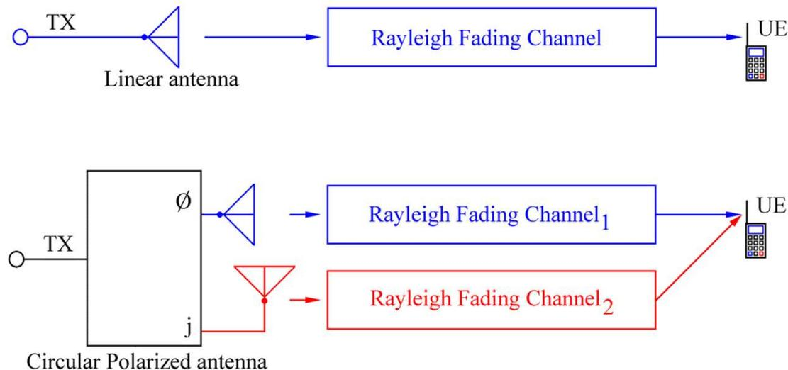
The diagram assume that the MTSO. is equipped with a linear cross-pole antenna, or a CPLPA. The UEs are, in both cases, assumed to be equipped with a single linear antenna.
